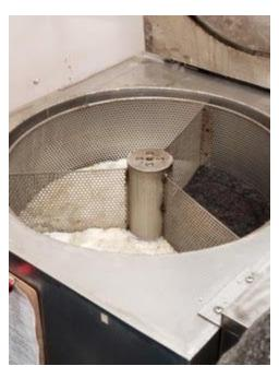
This is the machine that washes the fiber It can wash 3 different colors of fiber per load It is completely automatic, but unlike a household washing machine it does not
